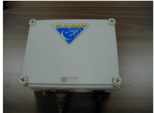
The Model 464-BC Monitor controls and stores flow data from Marsh-McBirney Flo-Dar sensors. A portable computer and Flo-Ware software is used to setup the flowmeter for the particular site and can also serve as a powerful data retrieval and reporting system. The three programmable 4-20 mA outputs provide a convenient way to transfer real time flow data to SCADA and other data collection systems, control systems and display devices.
